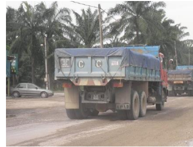
Lorry Covered with Tarpaulin during Transportation
